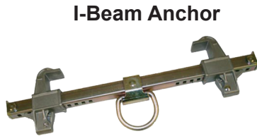
I-Beam Anchor Use Horizontally or Vertically Fits Width 3-1/2" to 12" with up to 1" Flange VV1B-1700
